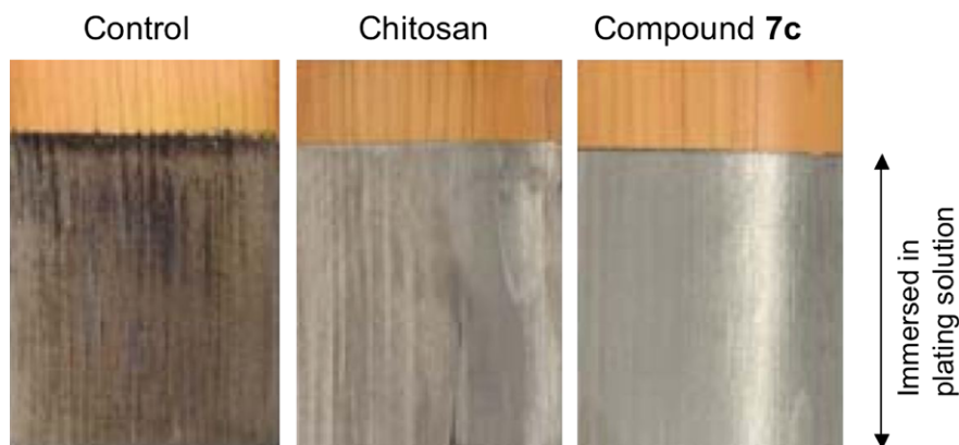
Fig. 7. Electroless nickel-plating on wood ( Japanese cypress ) coated by chitosan and UV-curable chitosan compound 7c .
